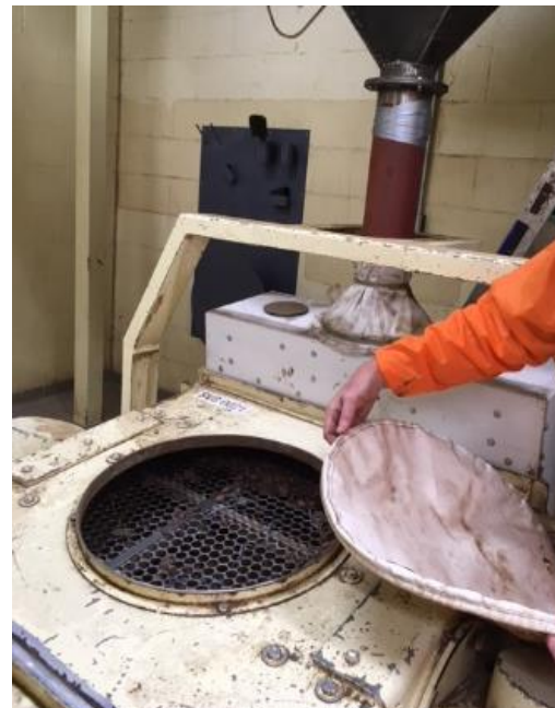
Further bean cleaning with inspection point grid and cover to protect entry of any further foreign bodies
