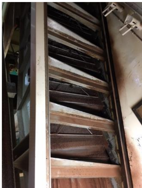
Sorting stairs used to grade the beans and remove variations in sizes of material passing through
