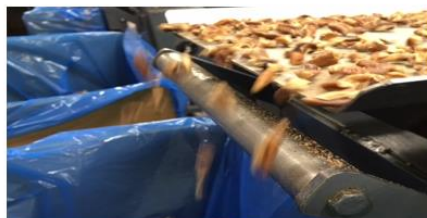
Magnets on Finish Line (removes metal burr)
