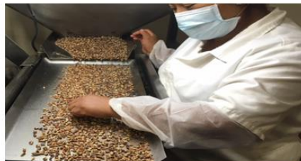
QA Table Inspection (inspect shell on the product according customer specs)
