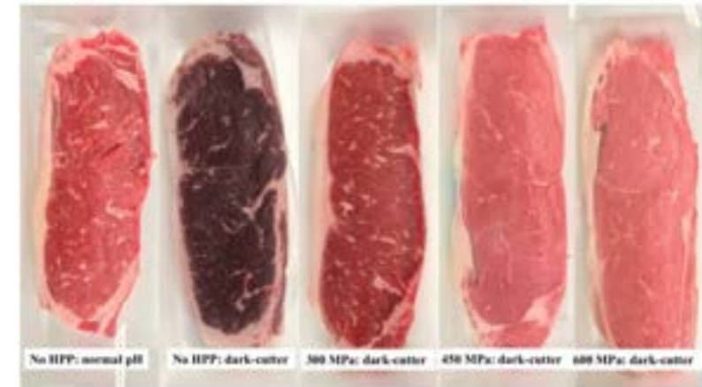
Effects of high-pressure processing (HPP) on surface color of dark-cutting beef on day 1 of display.
